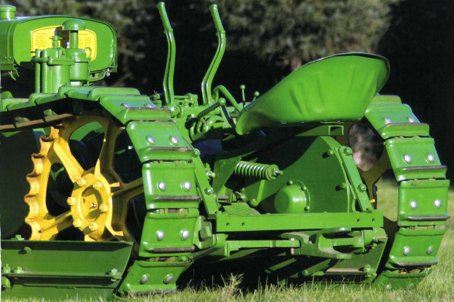
The GPO was steered through the manipulation of levers. Its transmission had three gears forward and one reverse.
