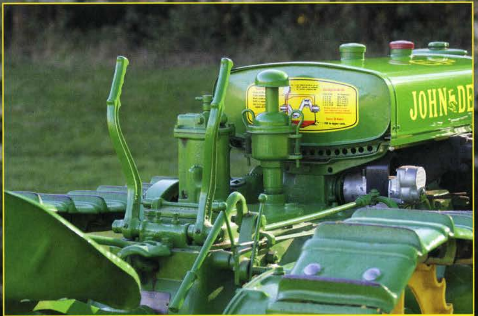
The GPO was steered through the manipulation of levers. Its transmission had three gears forward and one reverse.
