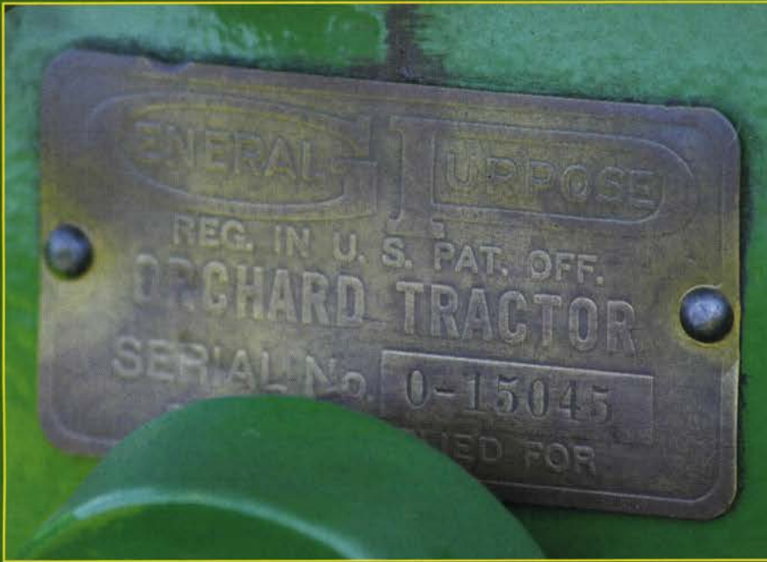
This tractor's original serial number tag shows "0-15045." It is the oldest John Deere GPO crawler known to exist in running condition.
