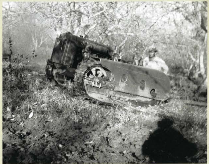
With their power, great traction, and low center of gravity, the Lindeman crawlers were well suited to the needs of orchardists in hilly country. Photo courtesy of Ted Adams and the Lindeman Archives
