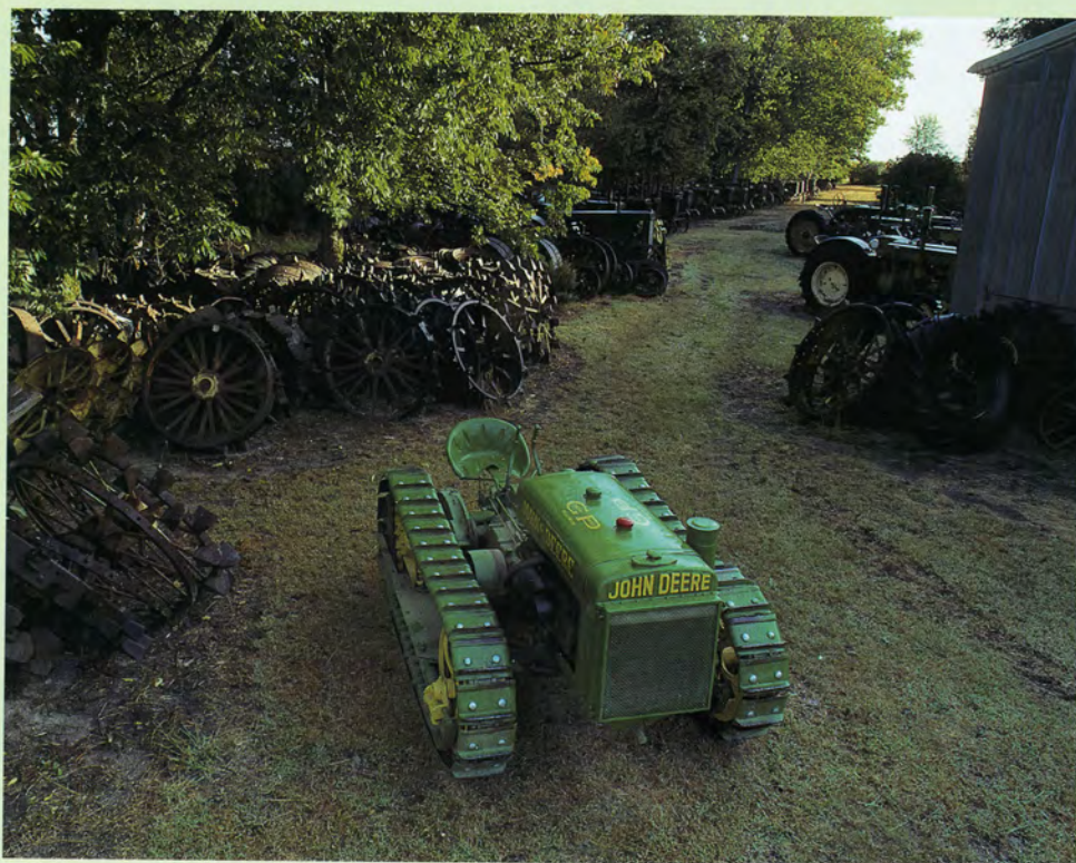
The John Deere GPO Lindeman-converted crawler became the second John Deere on tracks. This unit, somewhat popular for orchard work, also proved usable in some more traditional farm jobs. This model is one of the oldest ancestors to Deere's current popular bulldozer line. Randy Leffingwell
