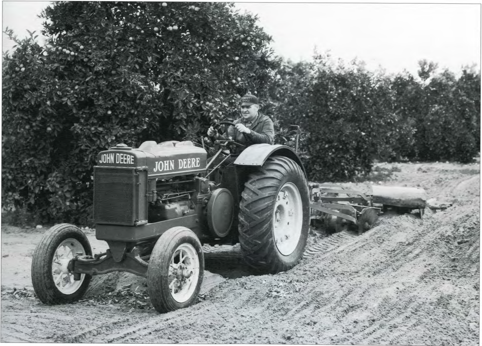
John Deere Model "BO" Tractor with disk harrow. The photo was taken in 1935 near Buena Park, California. An identifying feature of "B" Series Standard Treads, versus the "A" Series, is the center-located oval radiator cap. Note the protective shields over the air intake and in front of the fuel and gasoline caps, and the location of the ribs on the fender.
