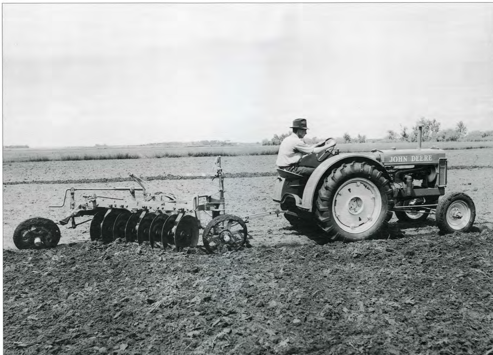
This early 1939 "BR" has the B1305R Cylinder Block with compression-relief cocks, but also has the flat-spoke steering wheel. This was the last year for the hump in the platform over the PTO, for the pressed steel wheels not having the four slots next to the rim, and for the wing nut on the seat bucket bolt. The implement is a No. 222 Disk Tiller.
