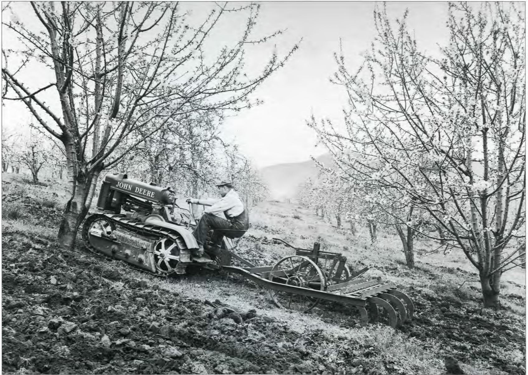
Lindeman-John Deere Model "BO" Crawler Tractor with 6-foot Killefer Chisel Plow. The terrain and often wet conditions were the inspiration behind the Lindeman Power Equipment Co. effort to develop a successful crawler attachment. The operator is identified as C.R. Chapman, Ashland, Oregon, May 1941.
