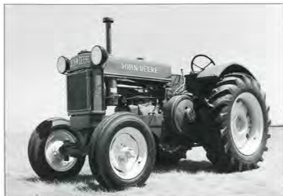
After the war, more "BR" Tractors were built with electric starting and lighting equipment. The slotted disc front wheels were adopted in 1940.
