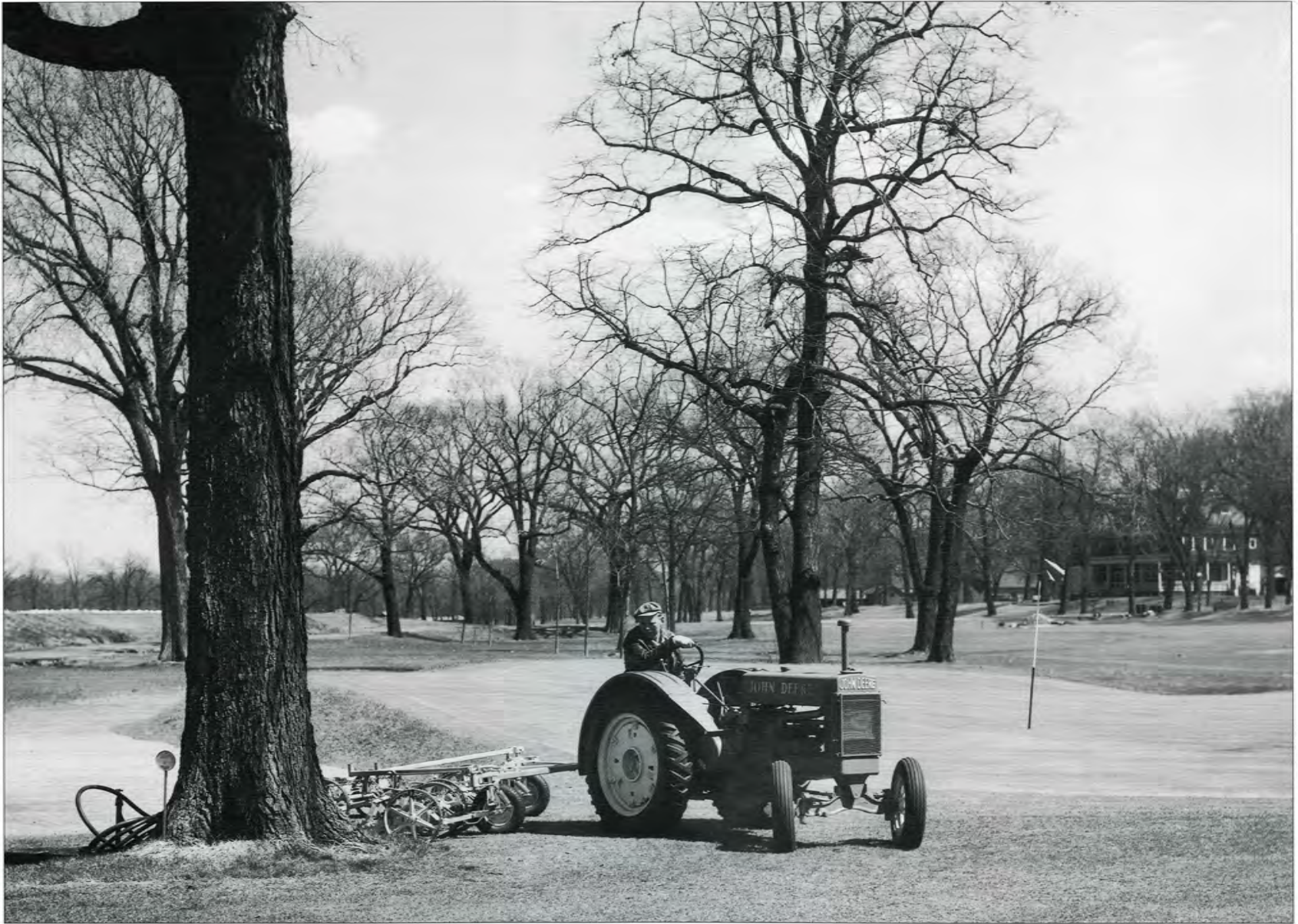
Although Model "BR" Tractors were intended to serve as the primary tractors on small grain farms or as the secondary tractor on larger farms, they were also a practical choice for applications such as golf course maintenance. This early unit (note the front wheels) is pulling a gang mower around the Arsenal Golf Course at Rock Island, Illinois, in April 1936.
