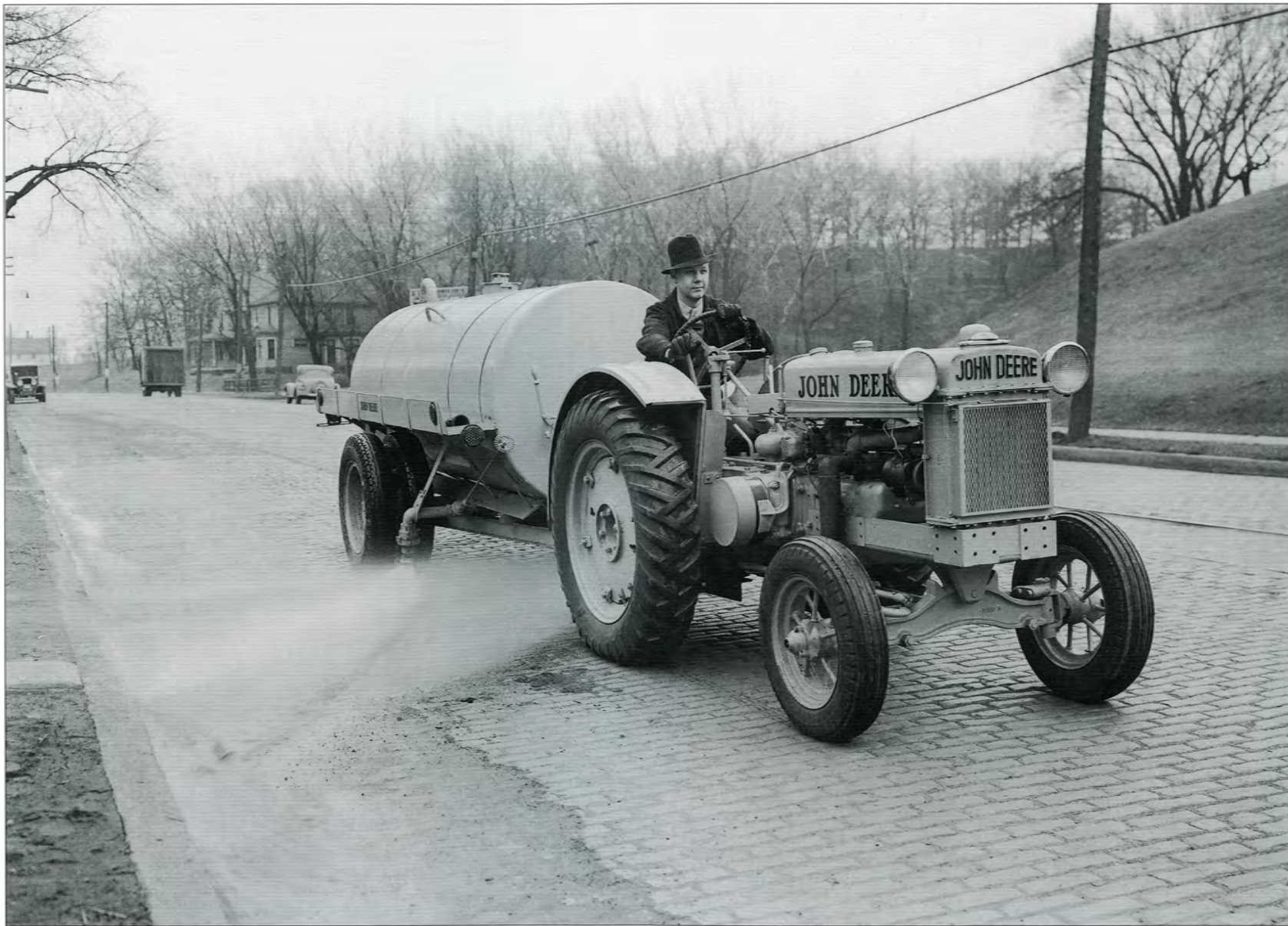
Rarest of the "B" Series Standard Treads, only 183 Model "B1" Tractors were built. Note the set-back front axle and machined front support (frame) of the tractor, as well as the industrial yellow paint job with black lettering. The equipment is a No. 30 Trailer with 1000-gallon Street Flusher.
