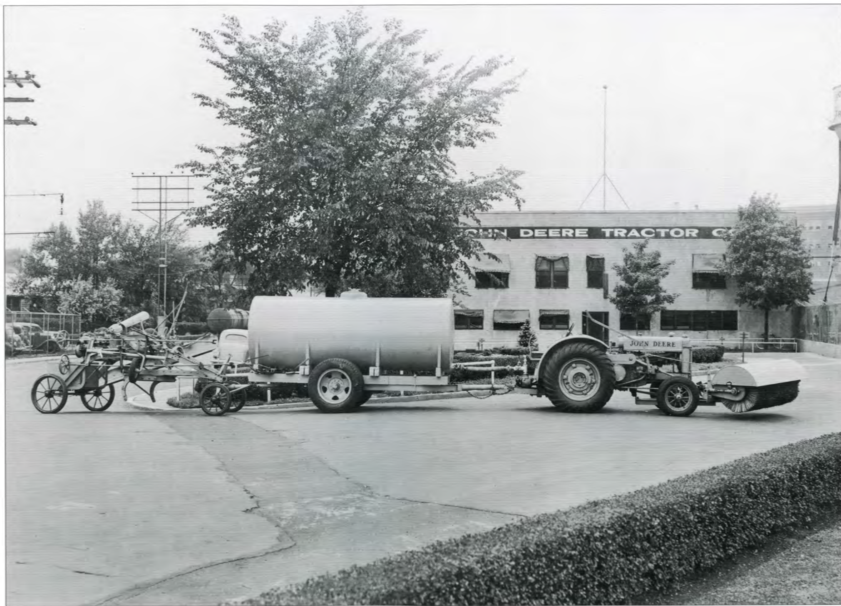
The "BI" shown here is equipped for display of several pieces of equipment normally used individually. From the front: Detroit Street Sweeper and Snow Brush, John Deere Street Flusher and Sprinkler Unit (mounted on the No. 30 Trailer), and a "Caterpillar" No. 4 Hi-Way Patrol (road grader).
