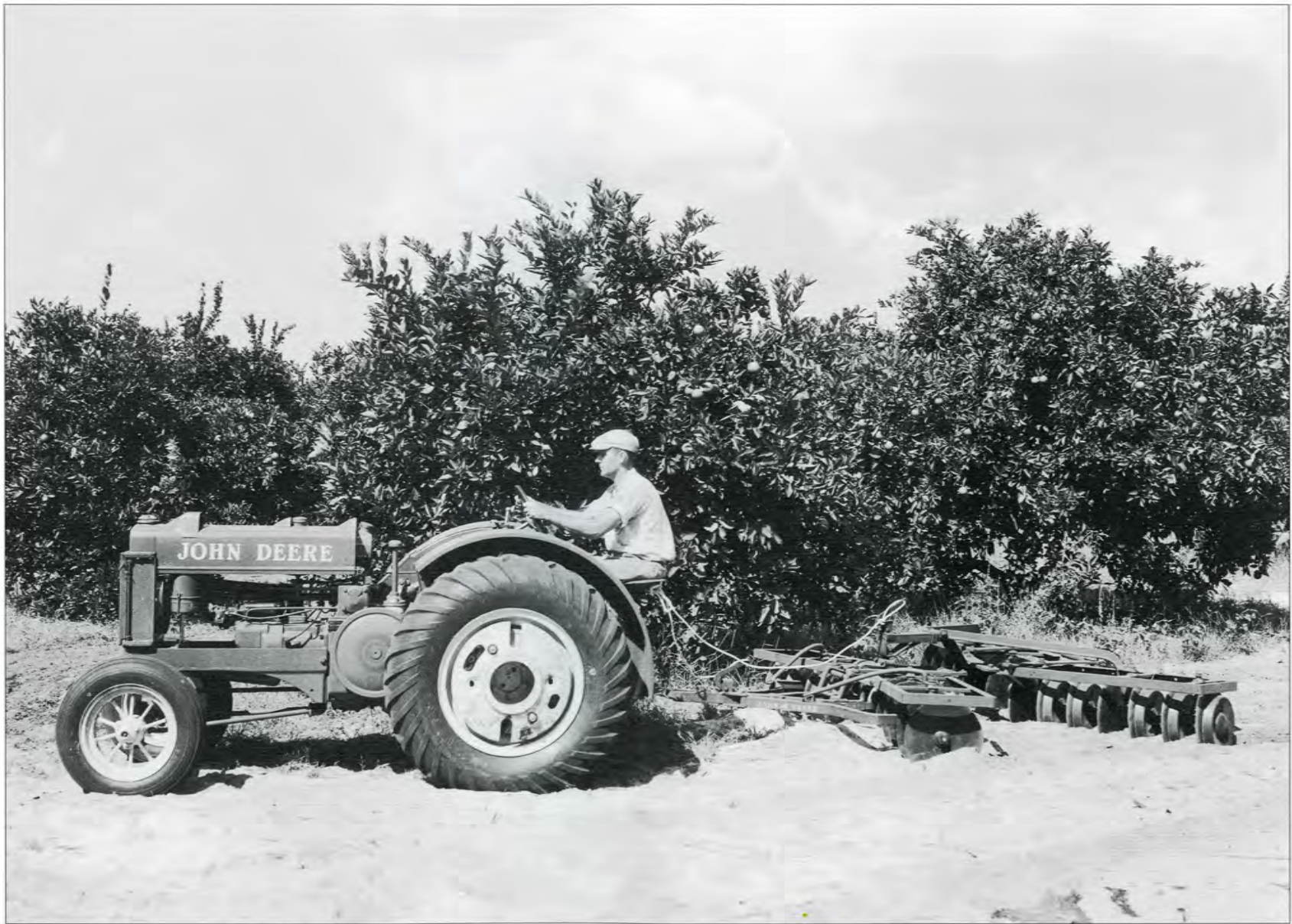
A side view of the tractor shown on page 4 shows the effective design of the shields, intended to keep branches from damaging or removing the protected parts. Although this photo was taken in Florida, conditions and crop are remarkably similar to those pictured in California on the preceding page.
