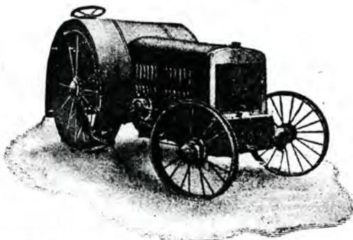
Rating 22 h. p.; 16 d. b.; 26 b. h. p.; 4 cyl.; 4 wheels; 2 drivers; speed 1½ to 6; 900 r. p. m.; pulley 9x7; front wheels 30x5; drivers 54x14; tanks, gasoline 25, kero. 25; cooling, radiator; length 87; width 52; height 60; weight 5,000; price \$1,250; bearings, Hyatt.
