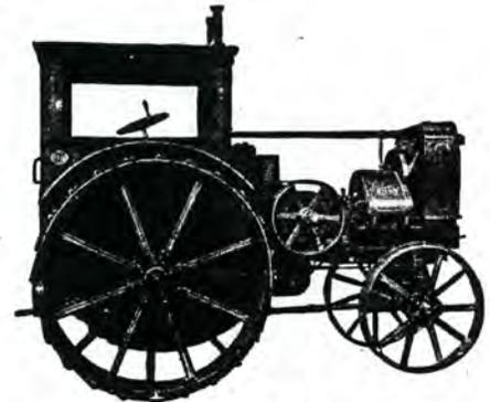
Rating 15-30 h. p.; 15 d. b.; 30 b. h. p.; 4 cyl.; 4 wheels; 2 drivers; speed 2.2-5; 575 r. p. m.; pulley 22x8; front wheels 40x7; drivers 66x14; tanks, gasoline 6, kero. 29; length 140½; width 85½; height 118; weight 9,580.
