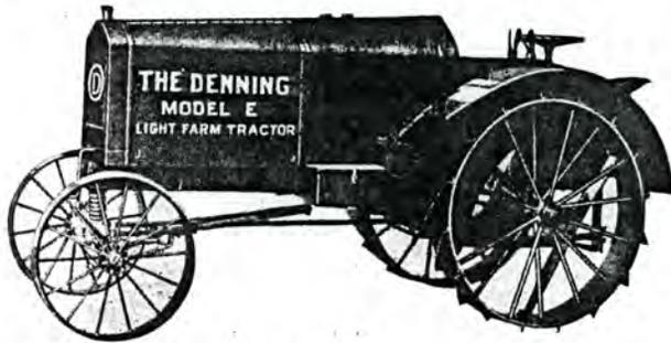
Rating 18 h. p.; 10 d. b.; 20 b. h. p.; 4 cyl.; 4 wheels; 2 drivers; speed  $1\frac{3}{4}$  to  $3\frac{1}{2}$ ; 1,000 r. p. m.; pulley 8x6; front wheels 30x5; drivers 46x10; tanks, gasoline 6, kero. 12; cooling, radiator; length 120; width 56; height 59; weight 3,600; price \$800; distributors—Owen Buxton Co., Chicago; E. E. Holland, Kansas City; G. H. Nichols, Fairfield, Neb.
