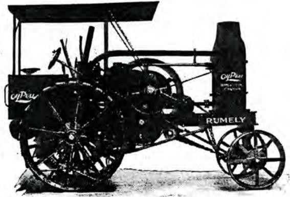
Rating 15-30; 15 d. b.; 30 b. h. p.; 1 cyl.; 4 wheels; 2 drivers; speed 2 to 2¼; 375 r. p. m.; pulley 30x9½; front wheels 38x12; drivers 70x24; tanks, gasoline 3, kero. 35; cooling, oil; length 192; width 94; height 123½; weight 16,500; price \$1,850; distributors as above.
