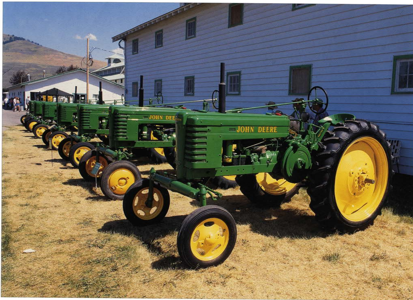
Eight of the featured Model "HWH" Tractors made it to the show, seven of them lining up here. Equipped with various options including extra-wide front axles, starter, lights, radiator shutter, and wheel weights, the tractors are owned by (right to left): Glen Knudson, Robert Lovegrove, Kimmelshue Brothers, Kenny Read, Jacob Rens, Chris Visser, and Doug Peltzer.
