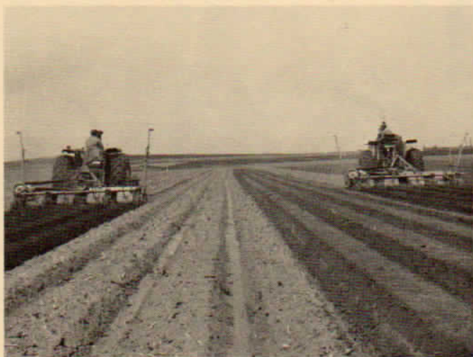
Here two 4 row Bedders retilling and reforming beds in a corn stubble field. The original beds were tilled and formed in the only previous operation.
