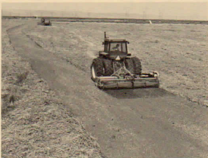
A Model "L" 12' Tiller is shown following the combine and is incorporating 110 bushel per acre wheat stubble to a depth of 8".
