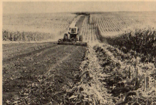
12' Tiller also following sweet corn harvester. Rib roller used in this quite sandy soil to prevent blowing.
