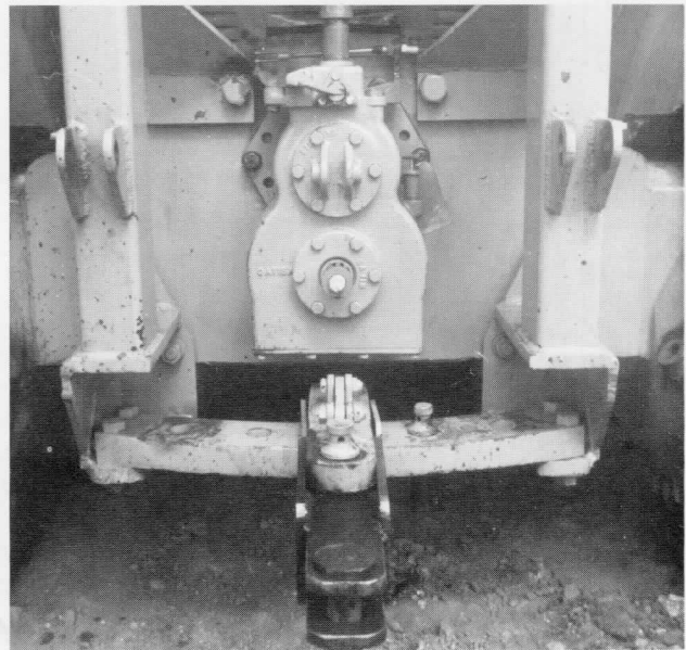
Close up of the NORTHWEST P.T.O. unit mounted on a D6.
