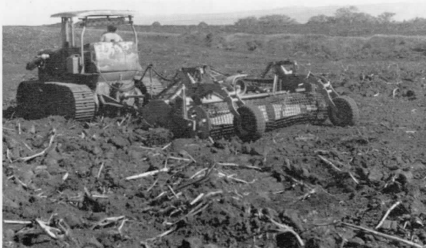
A Caterpillar D6 with the NORTHWEST P.T.O. operating a heavy duty tiller in a sugar cane field in Kauai, Hawaii.
