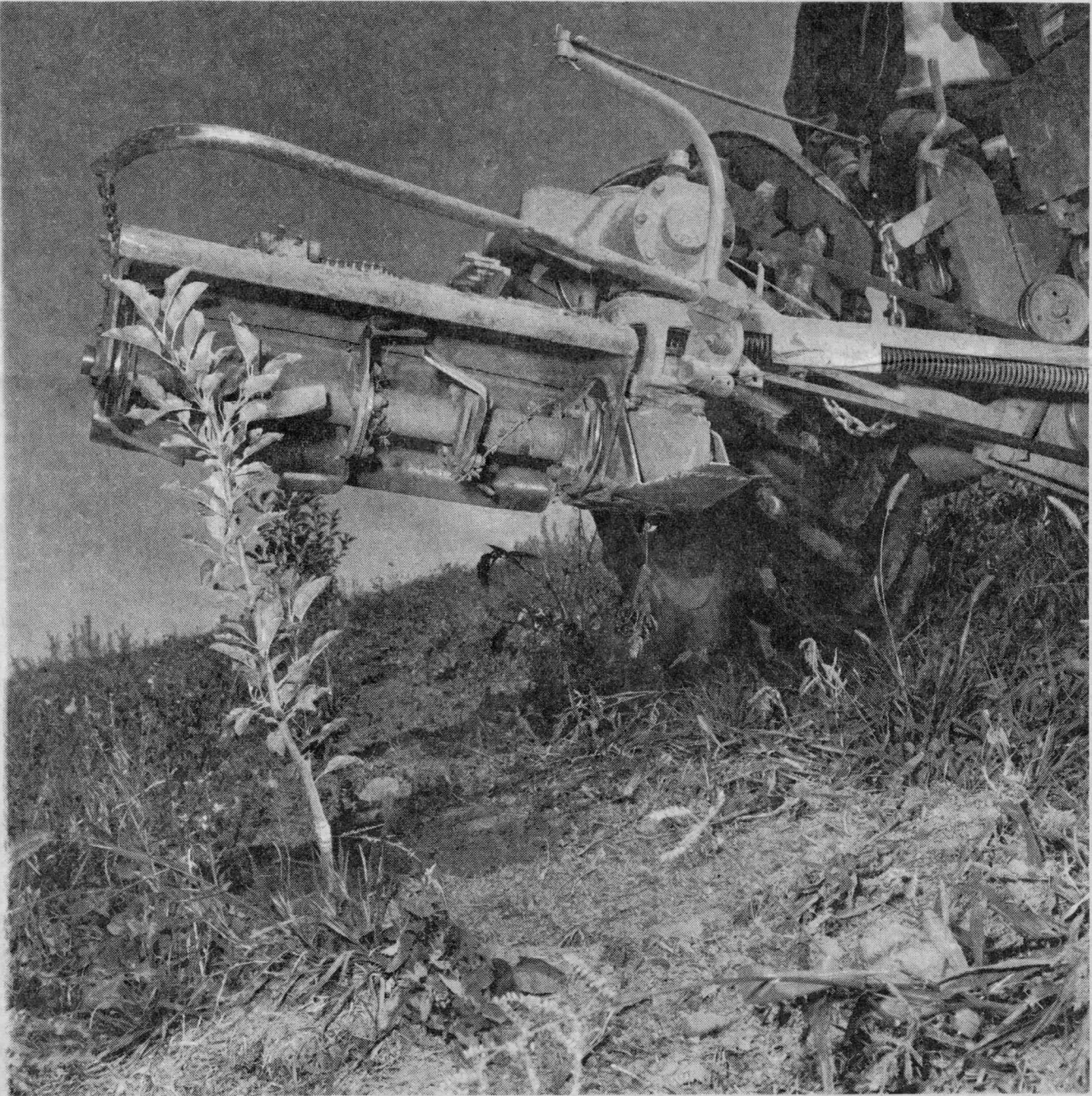
EASY CONTROL —Compact tractor-powered soil tiller is ideal for young trees in orchard. Rotating blades clear weeds and loosen soil around tree to depth of 1½-2 inches. Rod-like guard in front of unit activates a mechanism that folds tiller back, so it will slide lengthwise along side of tree instead of running over it. Bar is so sensitive it can be set to be activated by weed stems.
