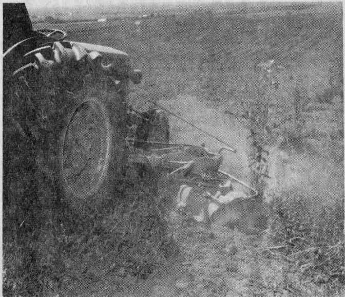
AT WORK —Mechanical weed tiller developed by Lindeman brothers of Yakima glided around young fruit tree in Wilbert Hansen orchard, on south slope of Ahtanum Ridge, without trace of injury to tree. Two such tractor-mounted units do weeding and tilling on 320 acres of new plantings for Hansen.
