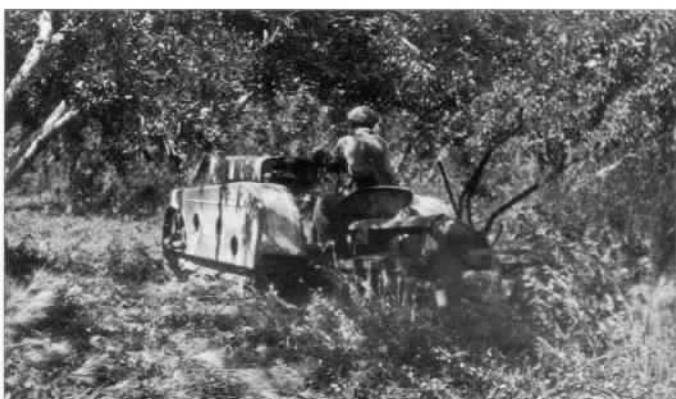
Top: With John Deere involved in producing "GPO" Tractors, the Lindemans wasted no time in testing the tractor with a crawler track attachment in place of wheels. The smaller tractor made far more sense than the "D" for grove and orchard use, and right at two dozen were built. Today they are highly prized by the few collectors fortunate enough to own one.
