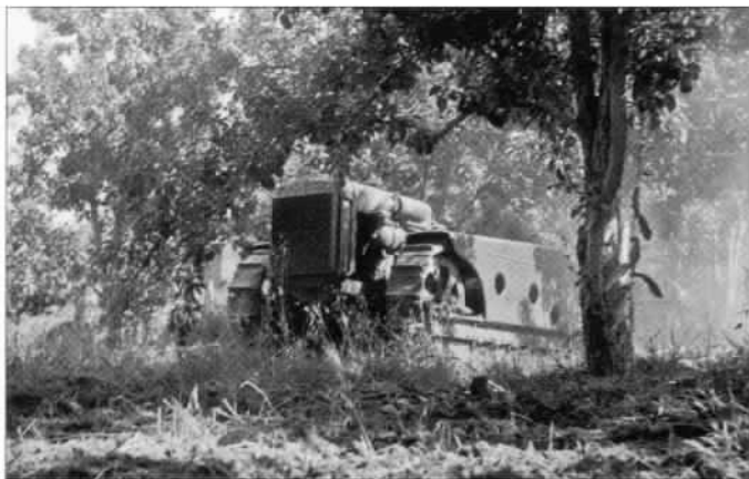
Top: With John Deere involved in producing "GPO" Tractors, the Lindemans wasted no time in testing the tractor with a crawler track attachment in place of wheels. The smaller tractor made far more sense than the "D" for grove and orchard use, and right at two dozen were built. Today they are highly prized by the few collectors fortunate enough to own one.
