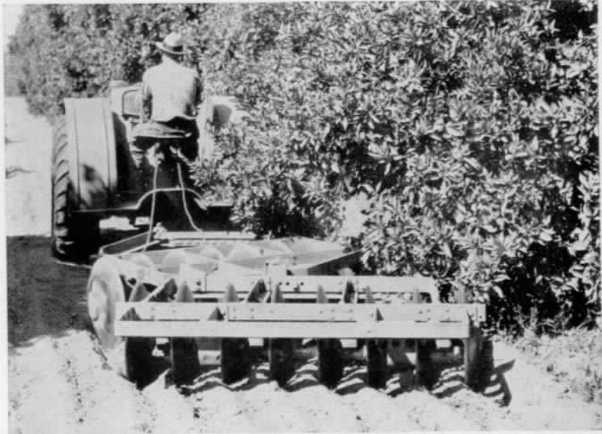
Here's a Model BO and Model OF Disk Harrow making a fine moisture-conserving mulch in a California pear orchard.
