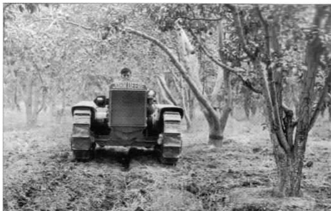
Top: With John Deere involved in producing "GPO" Tractors, the Lindemans wasted no time in testing the tractor with a crawler track attachment in place of wheels. The smaller tractor made far more sense than the "D" for grove and orchard use, and right at two dozen were built. Today they are highly prized by the few collectors fortunate enough to own one.
