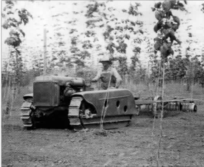
A full-fendered "GPO" Crawler doing a fine job of lightly disking a young grove of hops. Available information on the Lindeman-John Deere "GPO" Crawler seems to indicate that right at two dozen were built. Unfortunately, the cumbersome fenders have not survived with the handful-plus of known existing tractors.
