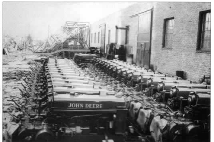
After everything was figured out, Lindeman ordered and Deere shipped "BO" chassis without the things not needed to build a crawler. The photo shows them lined up outside of the plant at Yakima, Washington.
