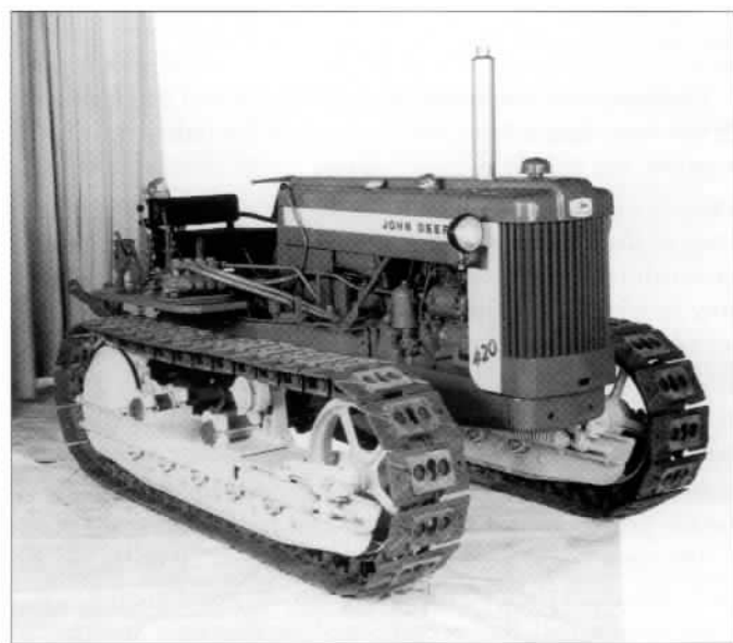
Studio photo of a five-roller "420" Phase II Crawler that is loaded with options: Three-point hitch, dual hydraulic system, street shoes, and direction reverser (the lever located near the rear of the hood).
