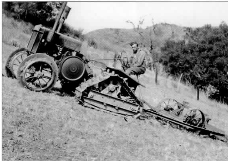
Ten of the 50 Experimental Exhibit “B” Model “D” Tractors (1930) were converted to half-track crawlers. This photo was taken near Havre, Montana.
