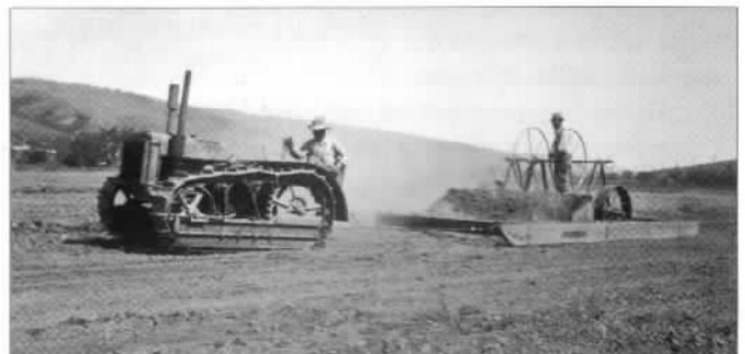
In 1932, the Lindeman Power Equipment Company developed a crawler attachment to be mated to the John Deere Model "D" Tractor. At least three "Ds" were converted by them to crawlers, and one was tested by Deere & Company. Here, a Lindeman-John Deere "D" Crawler is pulling a stone-boat type of land shaper, used to grade land for flood irrigation.
