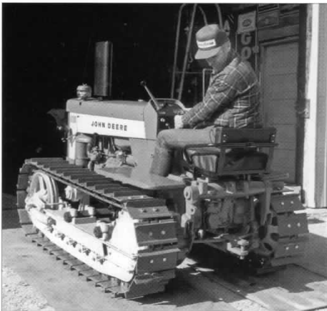
Top: Clearing a path with a "430" Crawler with headlight and grille guard, four-roller tracks (note sag in track, due to the absence of the track-support idler that came with the five-roller setup), and 62 Bulldozer. The special track shoes were for work in snow, and thus were called "snow tracks."
