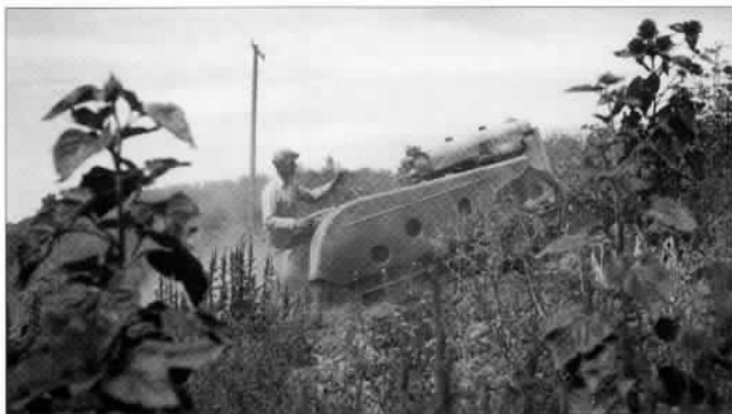
The advantage of the track system is clearly visible here with this Lindeman "GPO" Crawler in an uphill climb. When the "GP" Series was replaced by the "B" series, the Lindemans wasted no time in developing a crawler attachment for the Model "BO".
