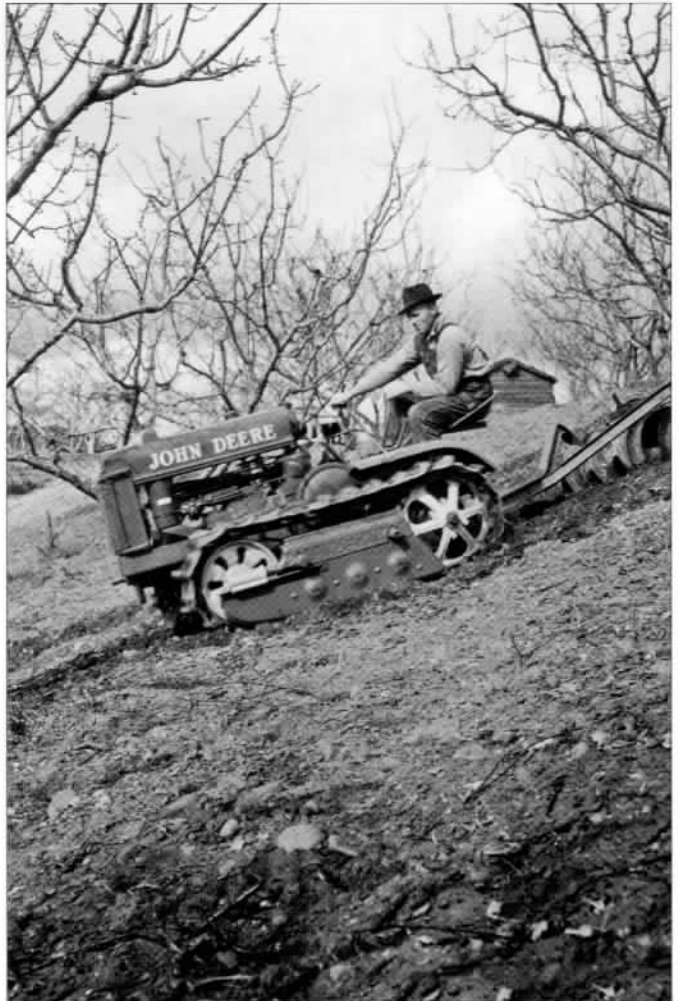
Starting in 1936, a new John Deere with tracks began to be seen in Washington's orchard country; the Lindeman-John Deere "BO" Crawler. Deere insisted that the "Lindeman" name preceded "John Deere." Note that "Lindeman" is not painted yellow on the track frame cover, a detail that most owners do not adhere to.
