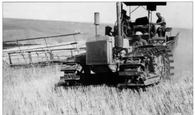
Stability, not speed, was the most important factor when pulling a hillside combine. In this photo, a Lindeman "D" Crawler modified with wide and deep grousers for better traction and stability on steep hillsides, is pulling a smaller model Holt hillside combine. The man with his hand on the steering wheel is responsible for keeping the combine level, while the other man fills and sews closed the sacks of grain.
