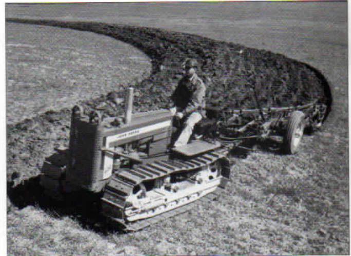
When John Deere advertised the "420" Crawler as having the capacity to pull three- or four-bottom plow, it wasn't an idle boast. A five-roller "420" Crawler equipped with grille and headlight guards is pulling a four-bottom 66-H Plow.
