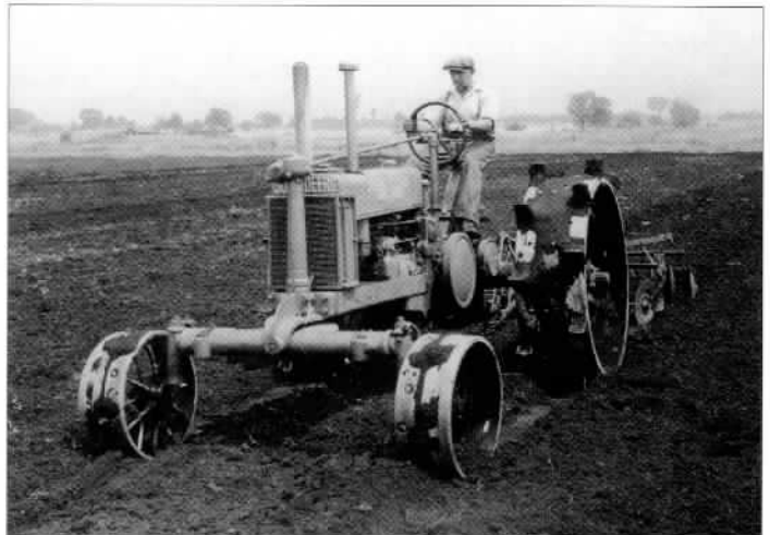
Model "B" of late 1935 or 1936 with early 1935 "BW" front axle. Collectors need to know how to spot conversions.
