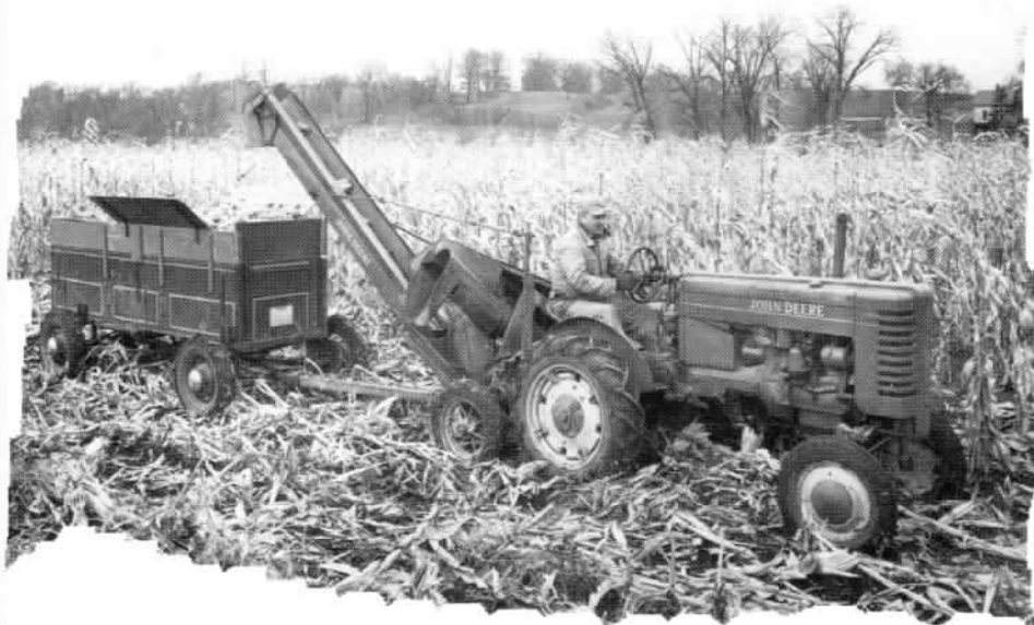
A 1944 "M" prototype: This one has a magneto and "H" style hydraulics. The door on the hood is for a gas starting tank for the all-fuel engine.
