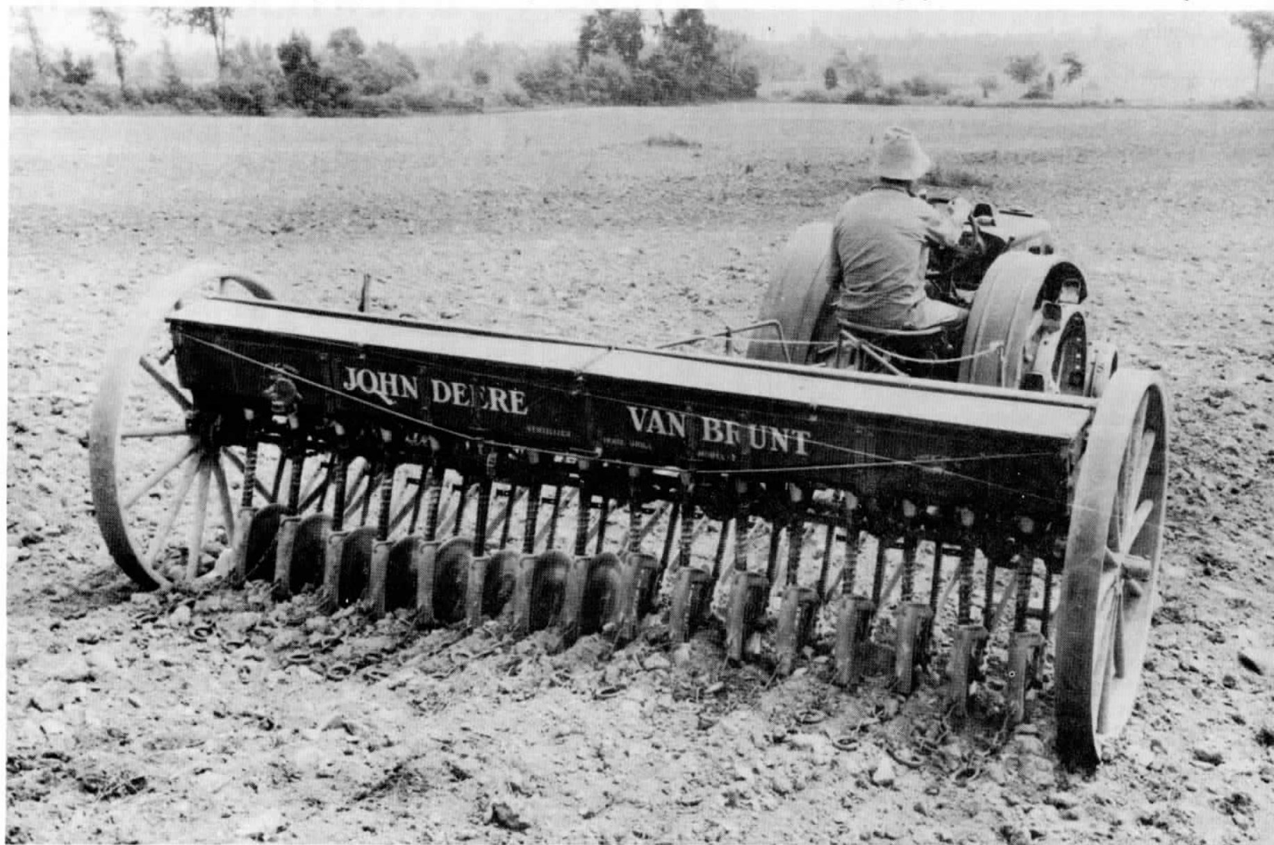
Model "BO" on steel pulling John Deere-Van Brunt Model F Grain Drill.
