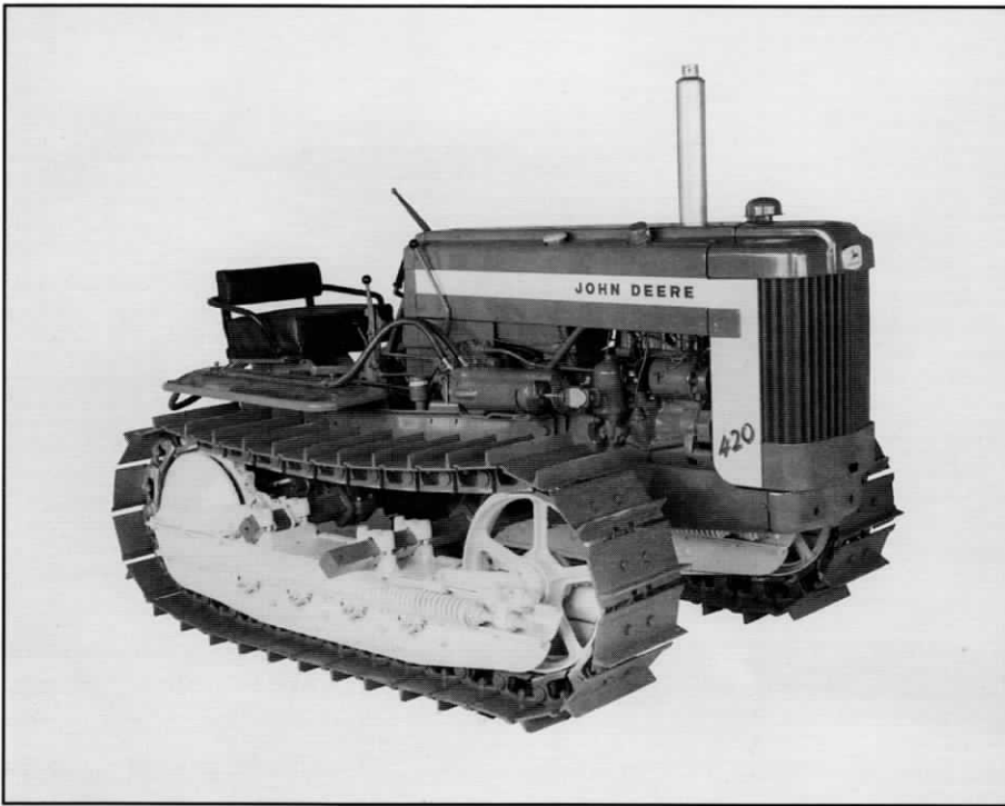
Studio photo of a Phase II 420 crawler, equipped with four roller track frame, single hydraulic system and direction reverser (tall lever next to hood. Note tracks are green.
