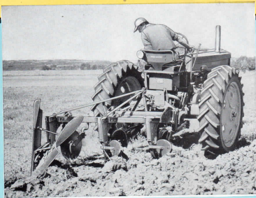
This three-bottom tool carrier plow is shown immediately after one bottom has hit a field obstruction.
