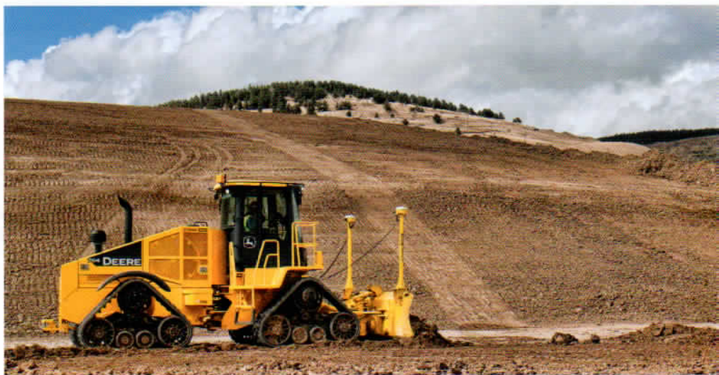
Above: The Deere-Lindeman crawler was first based on the Model "BO" Tractor until John Deere purchased Lindeman Manufacturing and started building its first crawler, the Model "MC." Right: The John Deere exclusive 764 High-Speed Dozer delivers speeds up to 16 mph — quick for a crawler.
