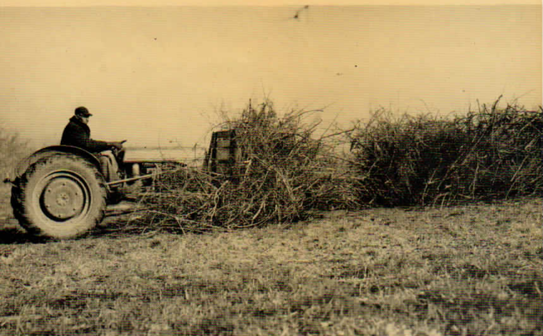
The Lindeman Brush Buck Rake mounted on the Ford-Ferguson Tractor gathers the limbs in the orchard and carries them to the brush pile where they are burned.
