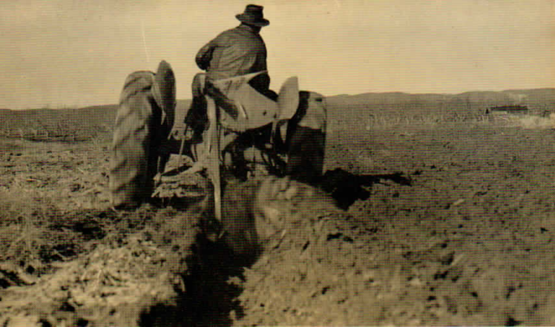
The Lindeman 2-way Plow for the Ford-Ferguson Tractor is especially adapted for complete plowing in confining areas.
