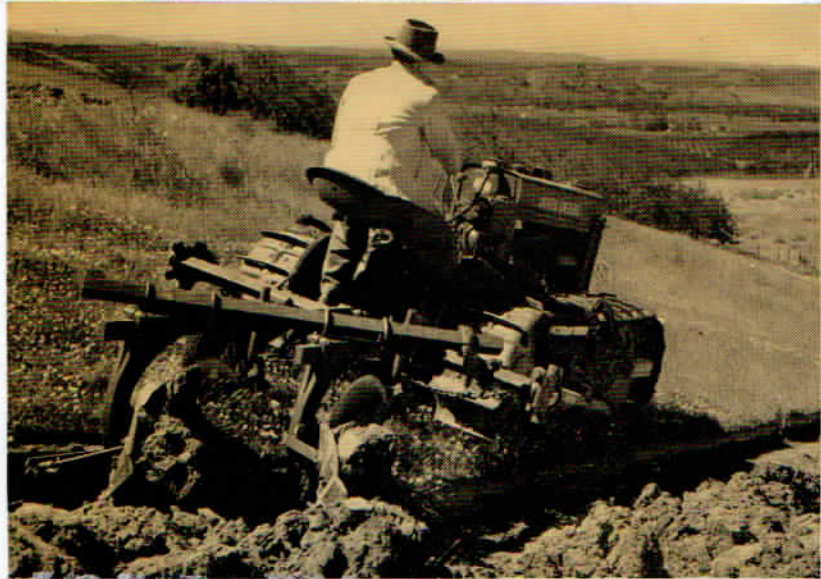
Difficult contour plowing is easily done with the Lindeman-John Deere Crawler Tractor mounted with the Lindeman Hydraulic Tool Bar and 2-bottom gang plow.
