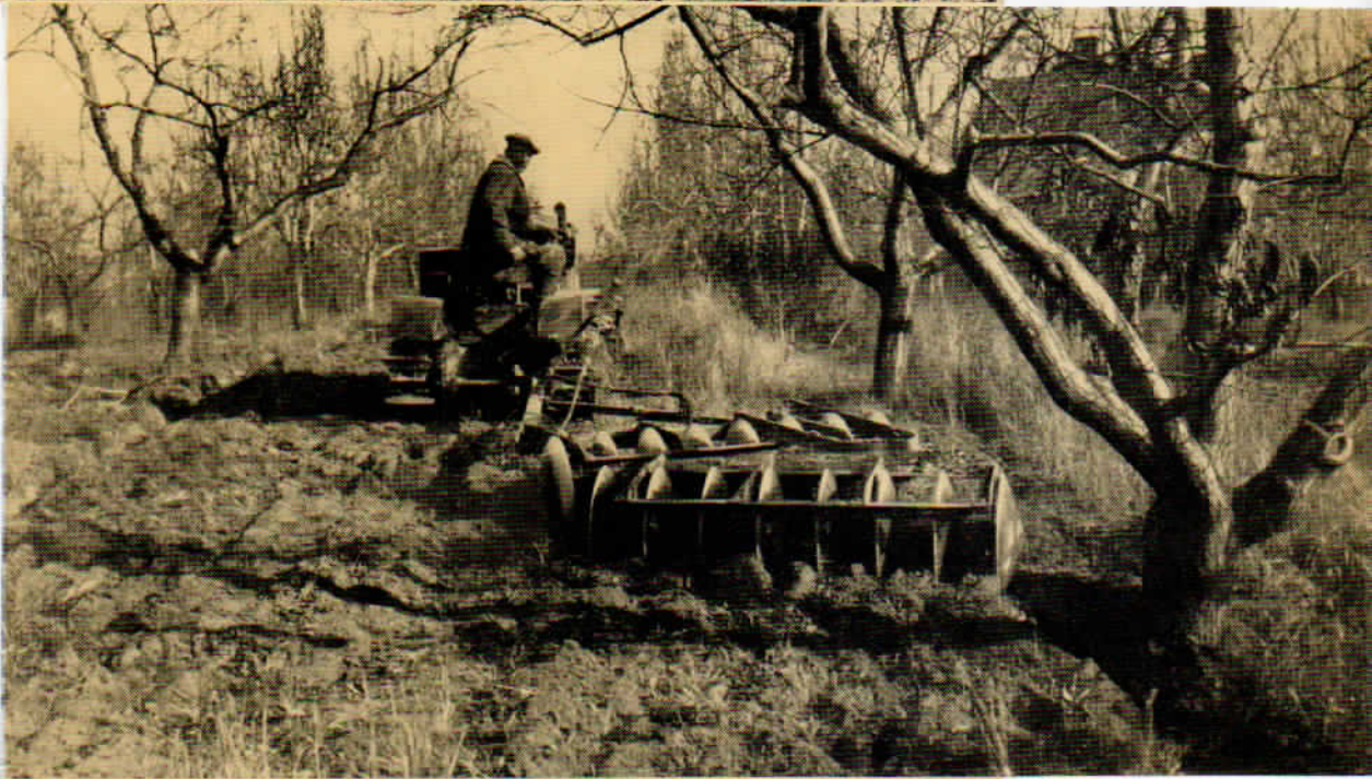
Cultivation close to trees without damaging limb, bark or roots is accomplished with the Offset Disc Harrow.
