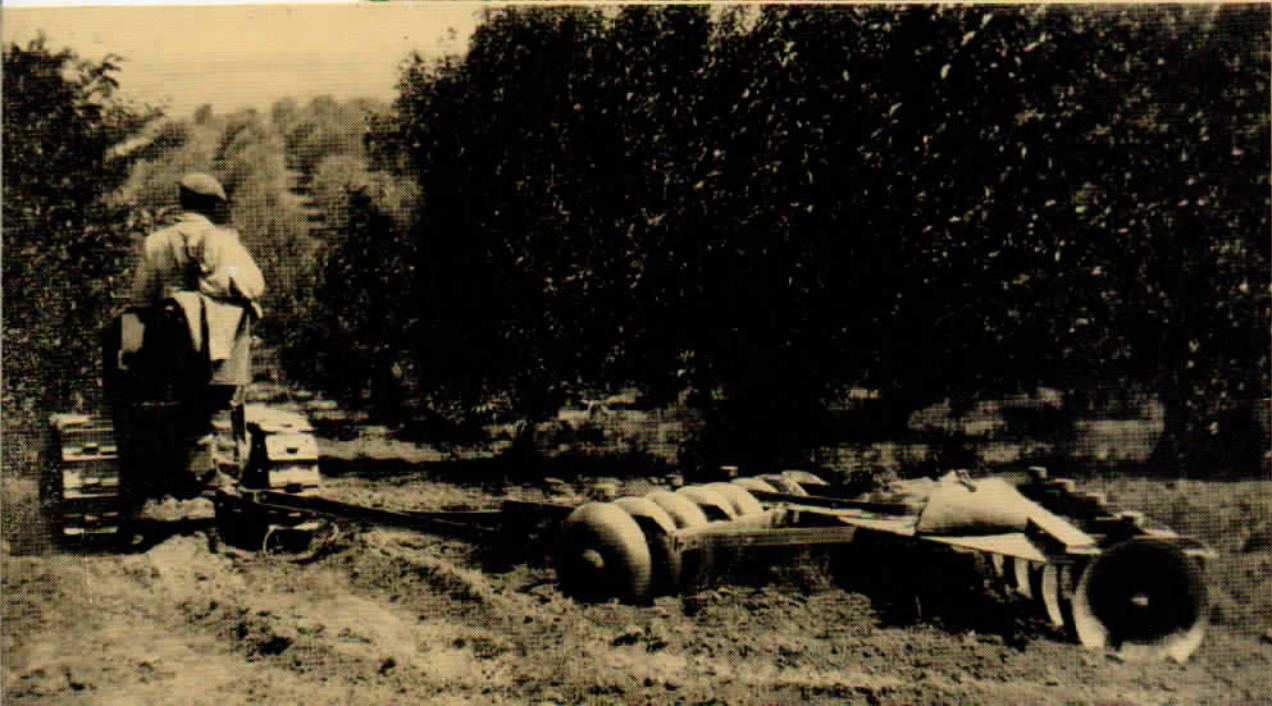
The Offset Disc Harrow with the Lindeman-John Deere Crawler Tractor makes a most maneuverable equipment unit.
