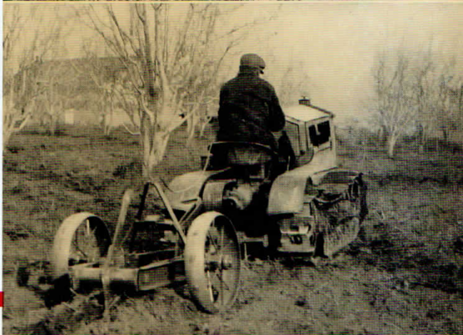
This Subsoiler which can not seriously damage pipe lines or roots was effective when used to curtail soil erosion and when preparing the seed bed in light soil.
