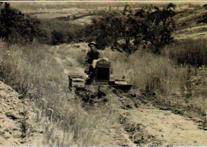
Lower left: With simple adjustments this Lindeman-John Deere Crawler Tractor with Lindeman Hydraulic Tool Bar and blade can be made into an effective angle dozer.
