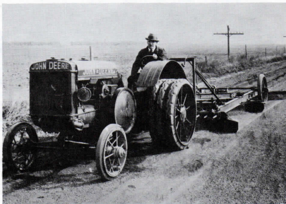
Grading with an early (circa 1926) industrial D. Note hard rubber tires.
