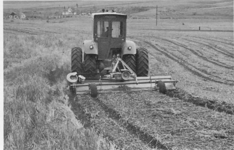
Heavy stubble from 115-bushel per acre Gaines wheat thoroughly mixed into five inches of top soil, above, in once-over operation of 12-foot Northwest Rotary Tiller produces erosion-resistant, smooth-surfaced field.
