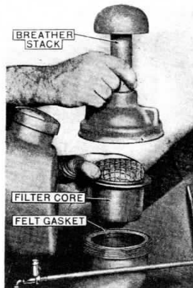
Removing Crankcase Breather Filter Core
