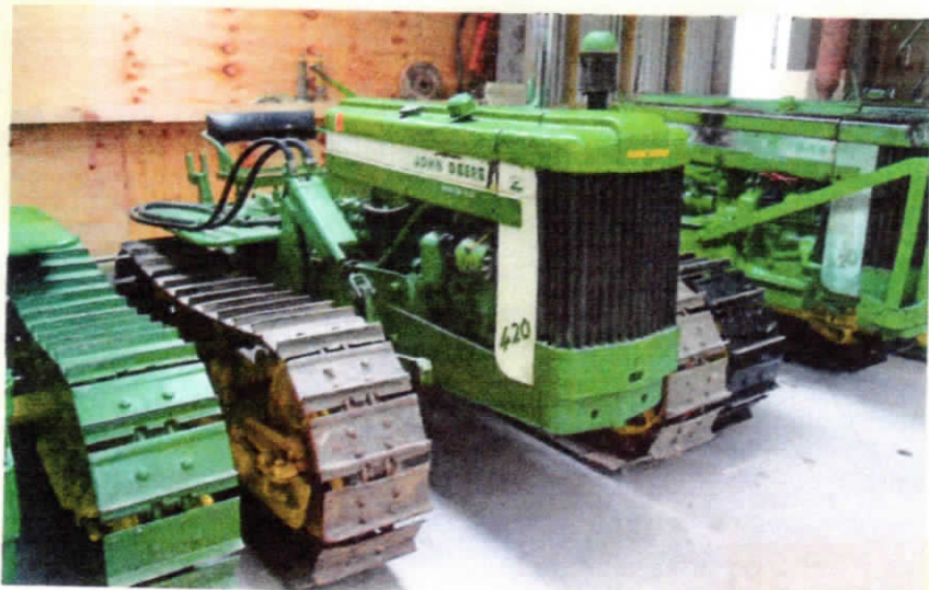
This particular 420 is fitted with hydraulic equipment for a bulldozer blade.
