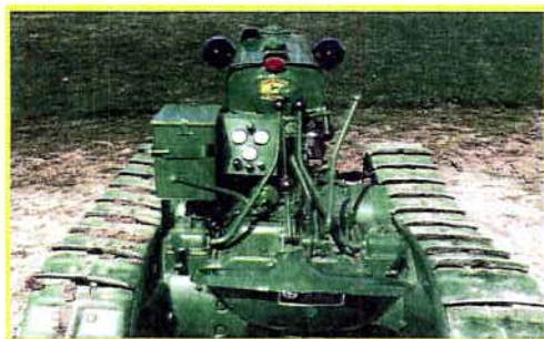
This view over the top (above) shows the crawler before Bill added the headlights. The location of the headlights, battery box and additional gauges.
