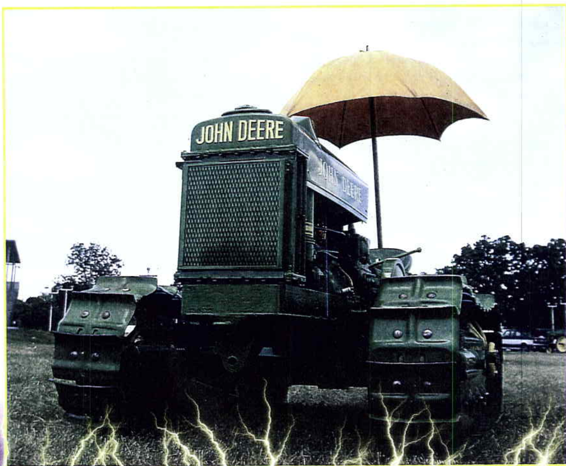
The pads, pins and fenders were replaced during the Lindeman's restoration.
