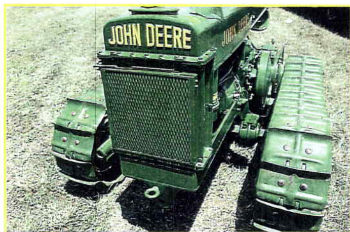
The shutters double as a radiator guard.
